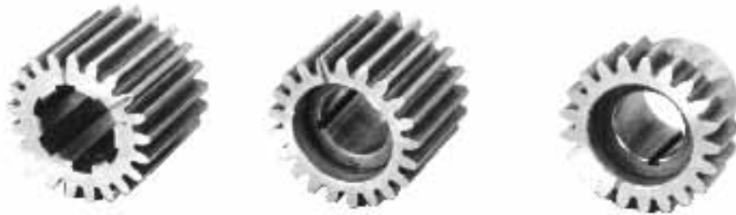
L-R: early, mid and late pinion gears
