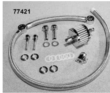
Sifton Braided Hose Crankcase Breather Kit Kit features a 3/8' I.D. braided stainless steel hose, breather filter with mounting stud, and hardware. Air cleaner and carb support bracket must be purchased separately. Fits 1993-2001 BT custom applications only. PCP Description 77421 Kit 77105 Breather 73500 Bolt kit
