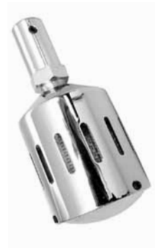
Sifton Braided Hose Crankcase Breather Kit Kit features a 3/8' I.D. braided stainless steel hose, breather filter with mounting stud, and hardware. Air cleaner and carb support bracket must be purchased separately. Fits 1993-2001 BT custom applications only. PCP Description 77421 Kit 77105 Breather 73500 Bolt kit
