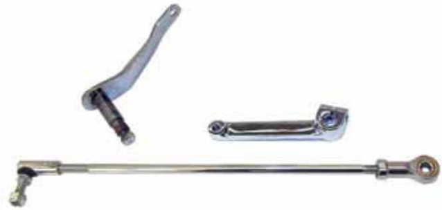
Chrome Shifter Arm and Linkage Kit Includes inner arm, inner shifter lever, and rod with ball and swivel ends. 36175 FXST 1986-on 36176 FLST 1990-on
